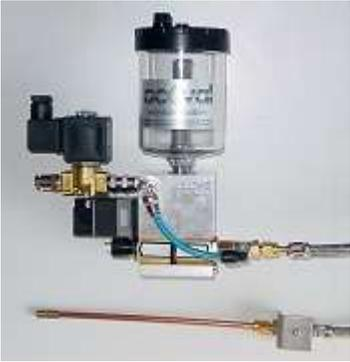
**Microlubrication** which is also named **minimum quantity lubrication (MQL)** is a means to bring **accurate quantity of liquid** in a process.
